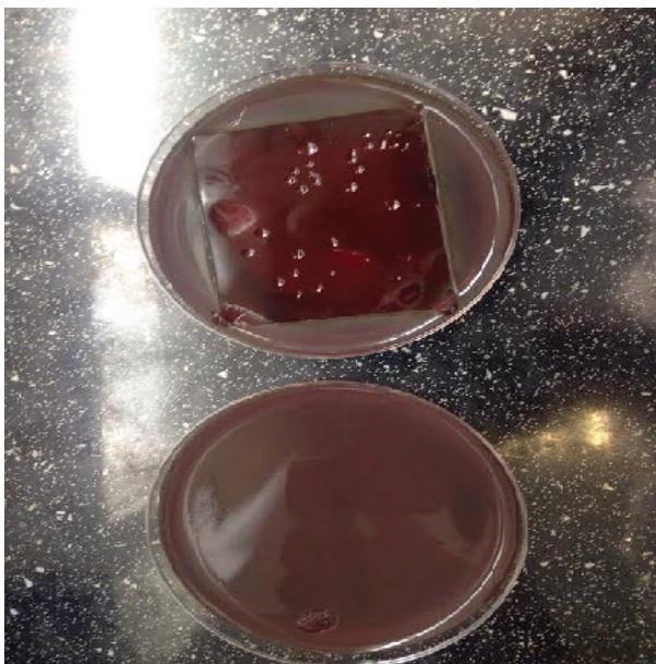
Figure 4. Biocide effect of copper strips after 24h of incubation; positive growth control with no copper strip
