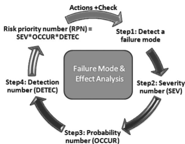
Figure 1. FMEA cycle (Hata *et al.* [3]).
