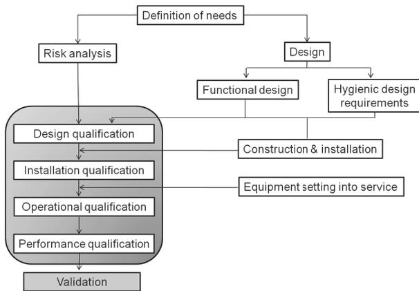
**Figure 1. The general process for qualification and validation of equipment. From the equipment manufacturer's perspective focus is on the four qualification steps: design qualification, installation qualification, operational qualification and performance qualification**
